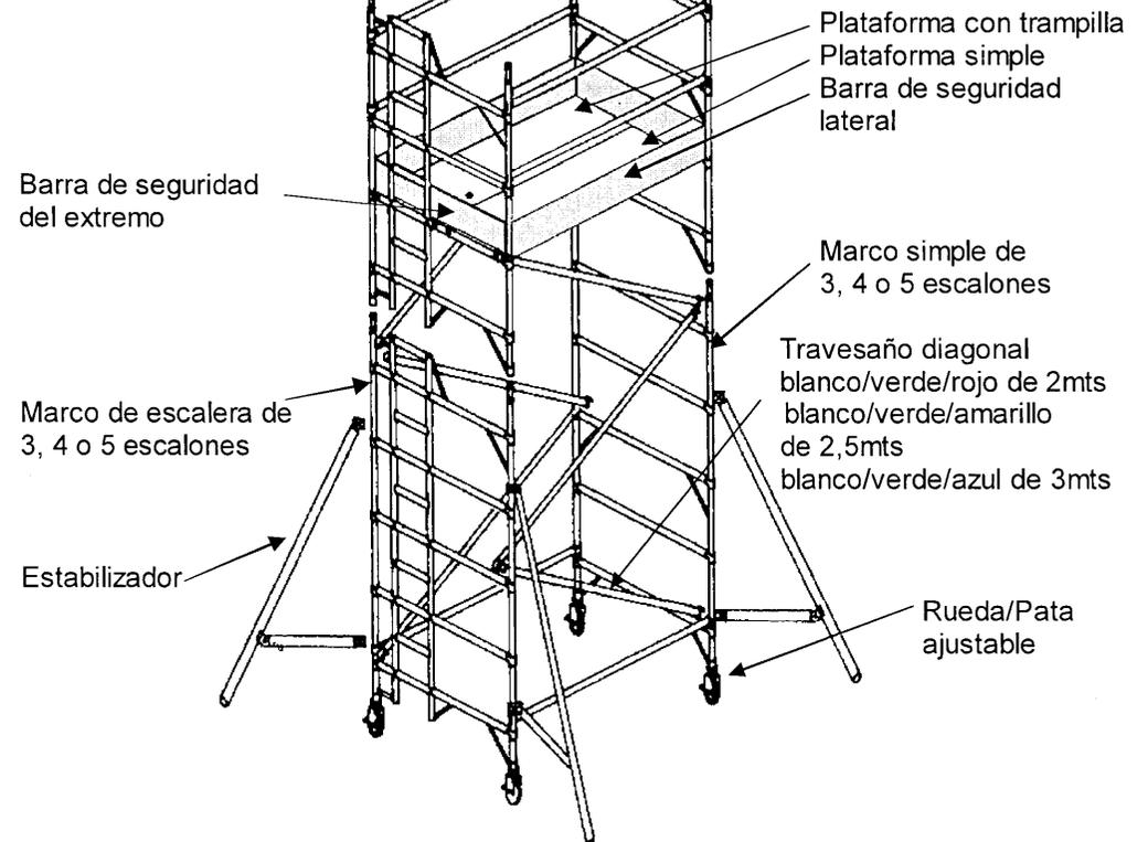
**CARGAS MÁXIMAS DE TRABAJO SEGURO PARA LA ESTRUCTURA: 750 KGS
